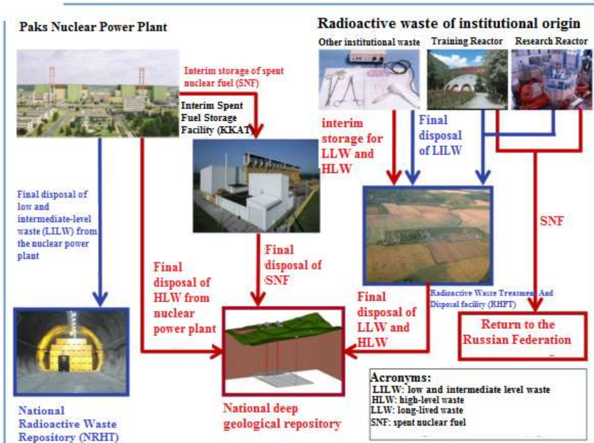
Figure 18: Logical scheme of the treatment of spent fuel and radioactive waste
