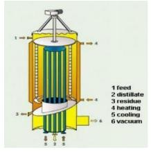
The film vaporiser (also called "thin film vaporiser) consists of 2 main assemblies:
