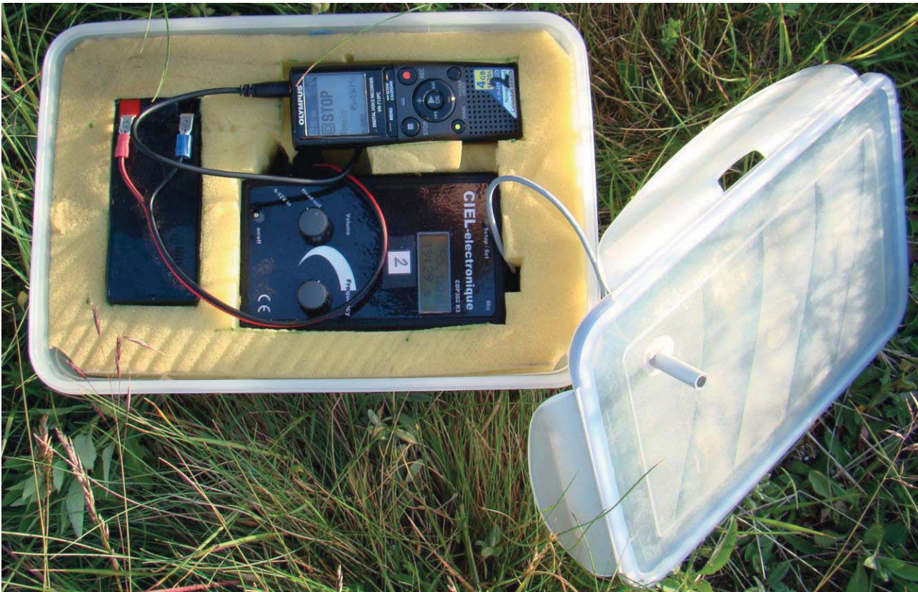
Figure 27. Automatic stationary bat activity detection system used in this survey. Photo: Ines Svenda, original.
