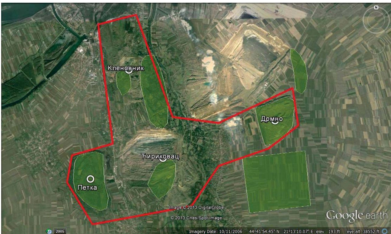
Figure 2. Potential wind farm development locations under the Nature Protection Institute of Serbia opinion (green areas). Source: JP EPS (General Design)
