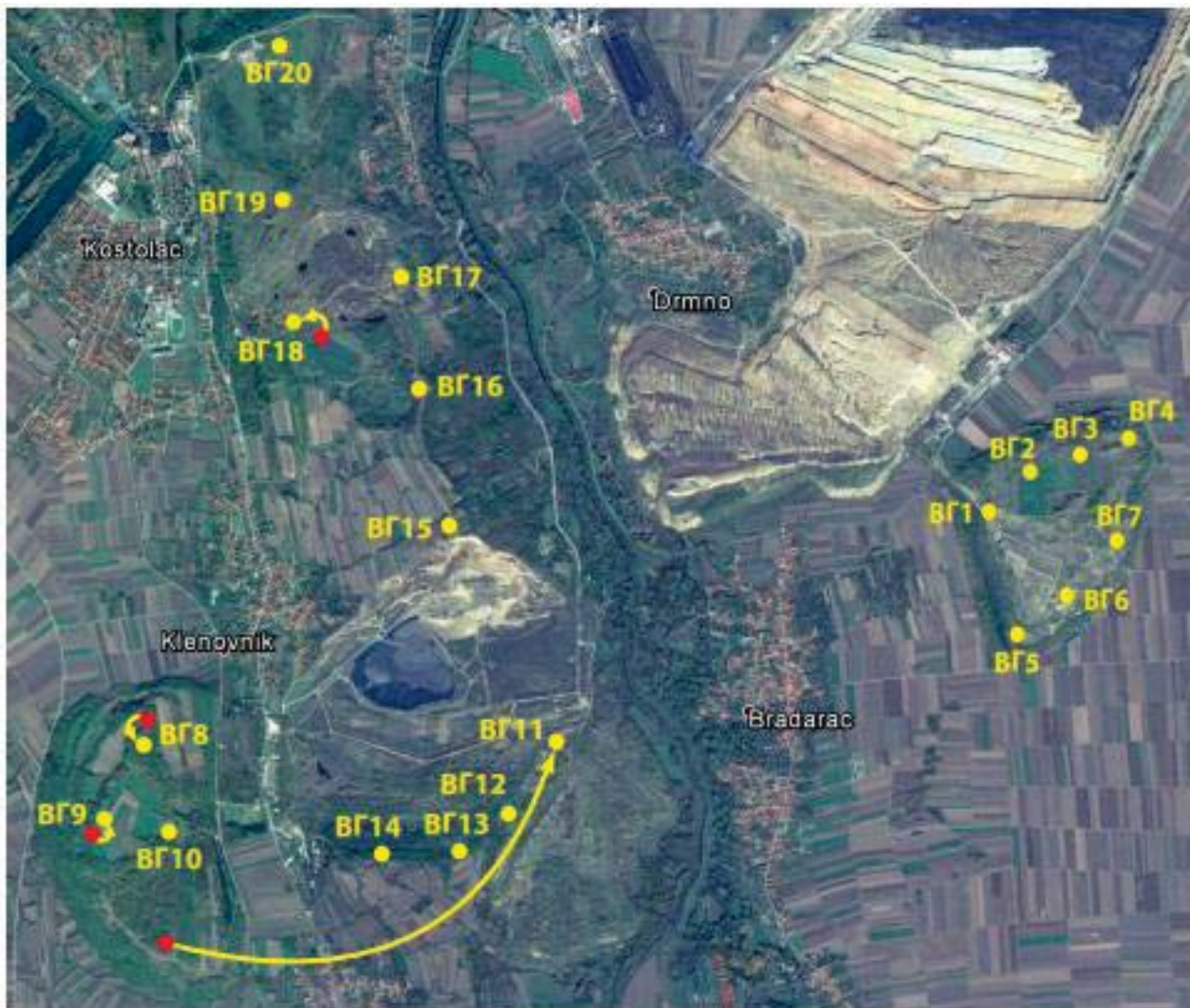
Figure 42. Changes to the wind farm plan as a result of the preliminary conflicts analysis at the start of this survey (red - wind turbines from the General Design, i.e. prior to the survey, yellow - wind turbine positions after the initial survey recommendations). Source: JP EPS and Google Earth 2014 Branko Karapandza, original.
