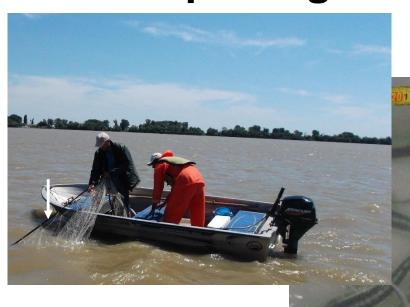
Fishing gear: bottom drifting trammel net
