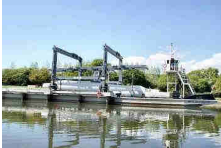
Figure 4.4. Barges with self-supporting crane for the transshipment of wind turbine equipment
