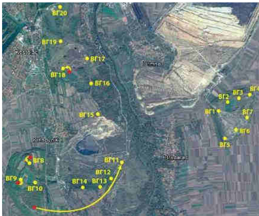
Figure 4.1. Changes in the spatial disposition of the wind turbines as a result of the analysis of potential conflicts with the flying fauna (red - the position of the wind generators according to GD, yellow - the position of the wind turbines after the conducted monitoring of the flying fauna)
