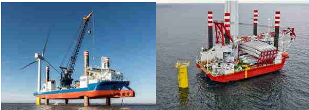
Figure 4.5. The ship with crane and supports mounting and transporting of wind turbines
