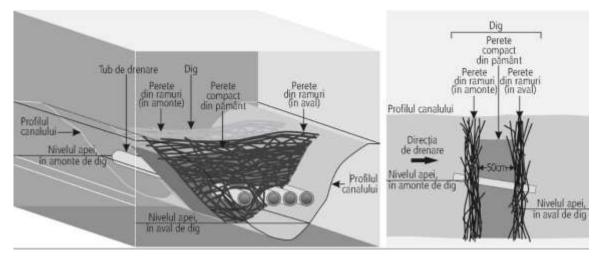
**Figure 2.** Diagram of a mixed dam constructed from natural and artificial materials (original)
