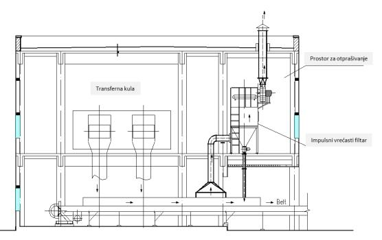
Figure 3.3.6-3: Scheme of the dedusting system in the limestone supply system
