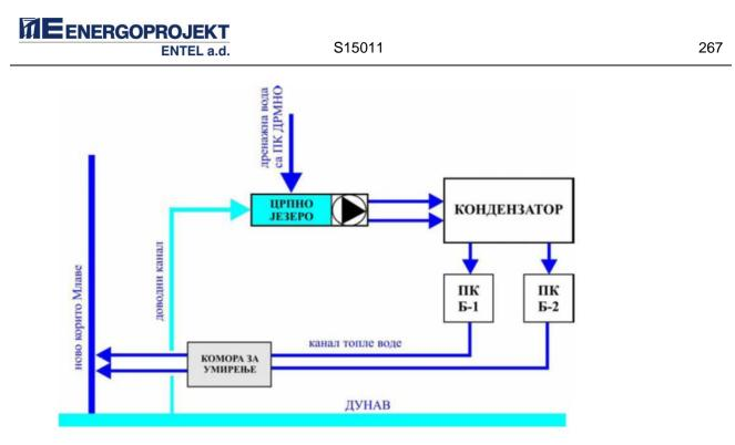
Figure 6.3.2-1: Cooling water flow scheme
