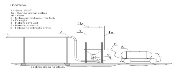
Figure 3.3.4-8: Scheme of silo for additive
