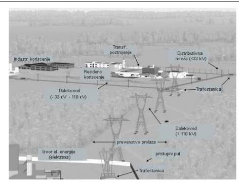
Fig. 3.3.5-9: Diagram of electric power transport from generation capacity to users
