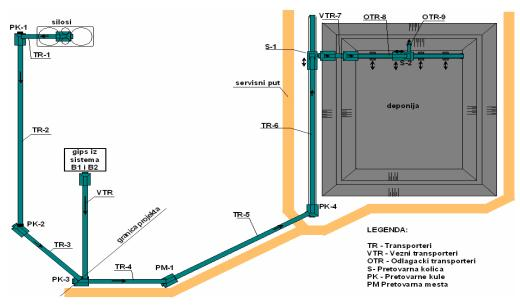
Figure 3.3.4-5: Scheme of transport and disposal of the mixture of ash, slag and gypsum
