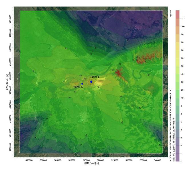
Figure 6.3.1-10: Spatial distribution of 99.73 percentille of NO<sub>2</sub> hourly concentrations in the vicinity of TPP Kostolac  $\,$  A and B,  $\mu g/m^3$
