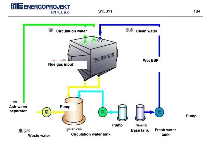
Figure 3.3.6-6: Principal scheme of wet ESP operation
