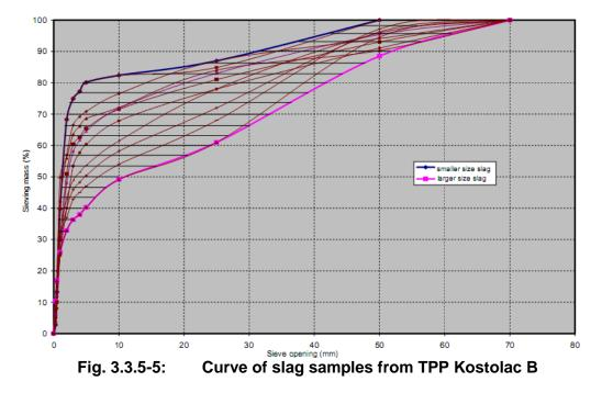
Provided results show that upper limit of slag particle size is in range from 50 to 70 mm, while mean grain diameter is from 1 to 10 mm, i.e. below 5 mm average.
