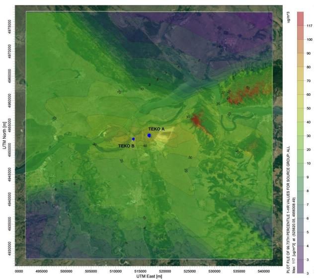
Figure 6.3.1-7: Spatial distribution of 99.73 percentille of SO<sub>2</sub> hourly concentrations in the vicinity of TPP Kostolac A and B, μg/m<sup>3</sup>
