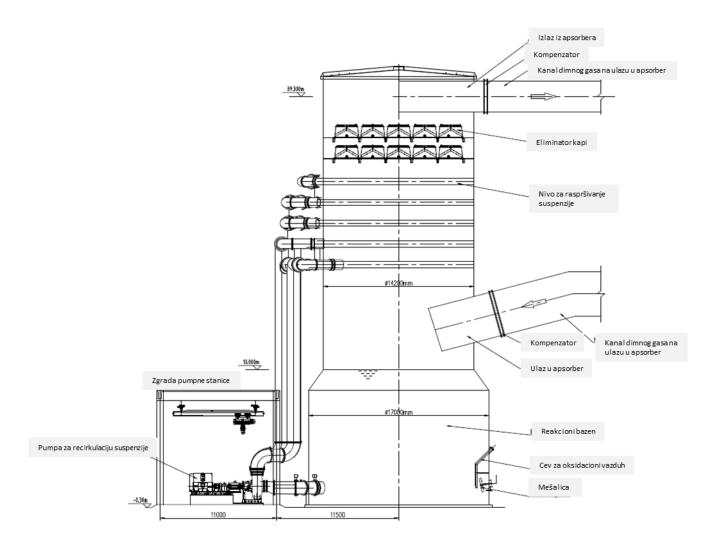
Figure 3.3.6-2: Absorber cross section
