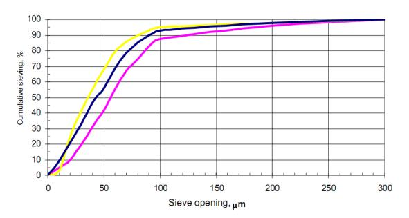
Fig. 3.3.5-6: Particle size composition of FGD gypsum
