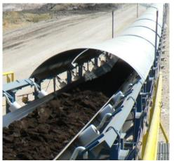
developed for covering the conveyor (conveyor for crushed coal in TPP Stanari)
