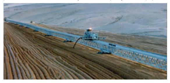
Figure 3.3.4-10: Spreading conveyor belt with tripper car
