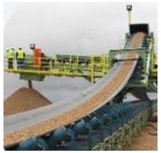
Figure 3.3.4-11: Tripper car with discharge belt
