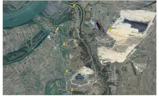
Picture 5.2-1: Measuring points of ambient air quality at the location of TPP Kostolac
