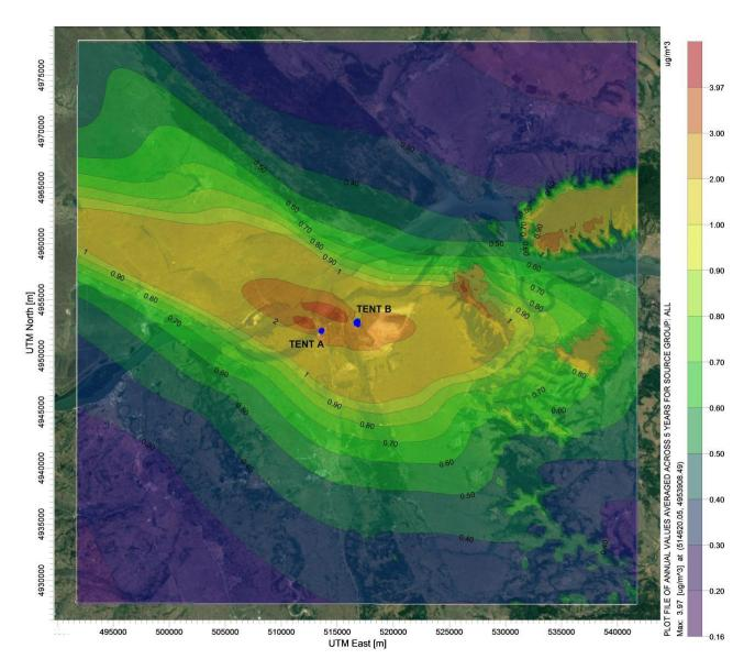
Figure 6.3.1-12: Spatial distribution average annual NO<sub>2</sub> concentrations in the vicinity of TPP Kostolac A and B,  $\mu$ g/m<sup>3</sup>
