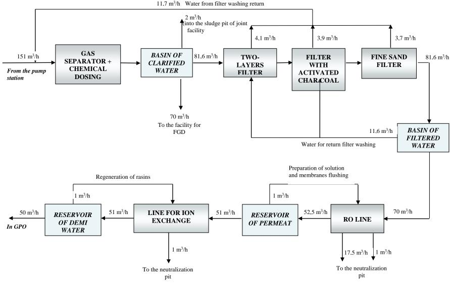
Figure 3.3.4-3: Balance scheme of the facility for chemical water treatment (one line in operation)
