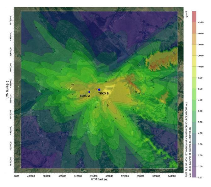
Figure 6.3.1-11: Spatial distribution of maximum daily NO<sub>2</sub> concentrations in the vicinity of TPP Kostolac A and B,  $\mu$ g/m<sup>3</sup>
