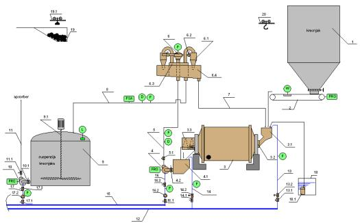
Figure 3.3.6-4: Principal technological scheme of limestone grinding
