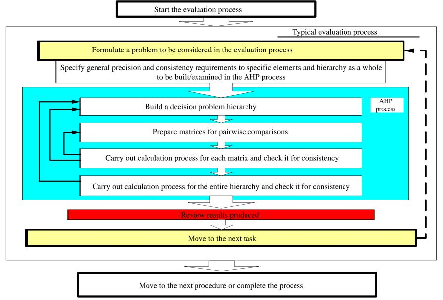
Figure 4.7. Process Flowchart: Comprehensive Environmental Impact Assessment Process Based on the AHP Method
