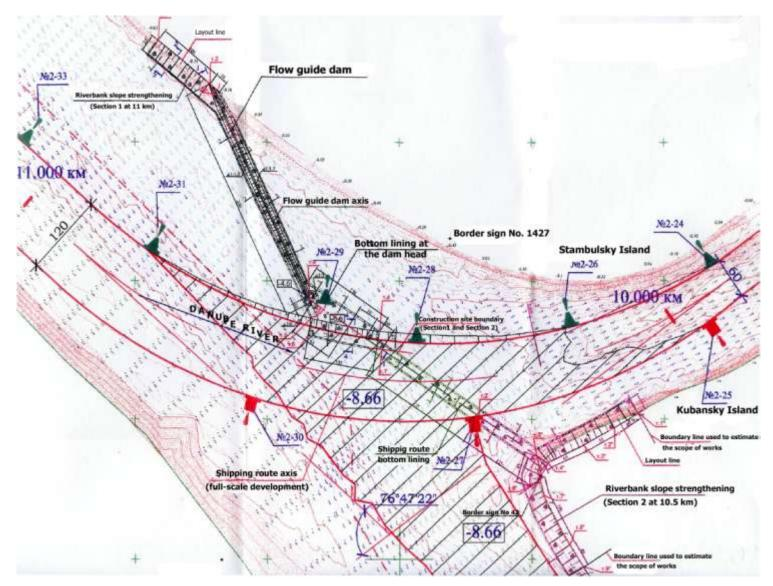
Figure 3.7. Flow Guide Dam and Strengthened Riverbank Sections at the Bifurcation of the Bystre and Starostambulske Branches
